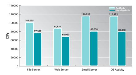
Figure 4: FastPath vs. Non-FastPath Real Work Performance
