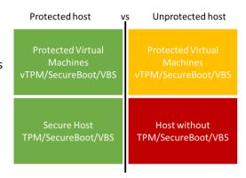
VBS uses hardware virtualization features to create and isolate a secure region of memory from the normal operating system. Windows can use this "virtual secure mode" to host a number of security solutions, providing them with greatly increased protection from vulnerabilities in the operating system, and preventing the use of malicious exploits which attempt to defeat protections.
