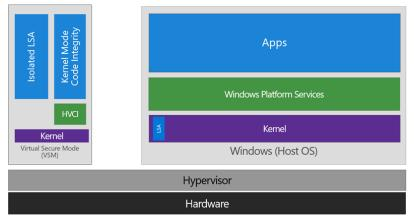
One such security solution example is HVCI, which uses VBS to significantly strengthen code integrity policy enforcement. Kernel mode code integrity checks all kernel mode drivers and binaries before they are started and prevents unsigned drivers or system files from being loaded into system memory.
