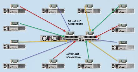
Alternatively, the dual PCI-E 3.0 x16 slots can support dual NVMeoF add-on-cards to enable additional deployment scenarios.
