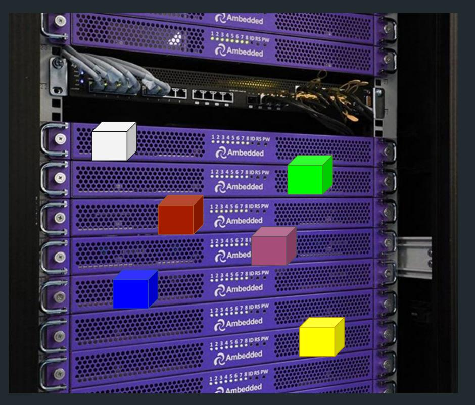
K+M = 4+2, Allows max. 2 chassis failures Capacity consumed is (K+M)/K of original data
