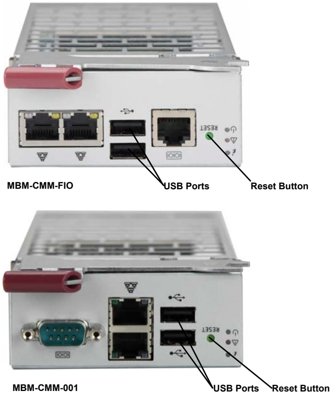
Figure 4-7. USB Ports on CMM
