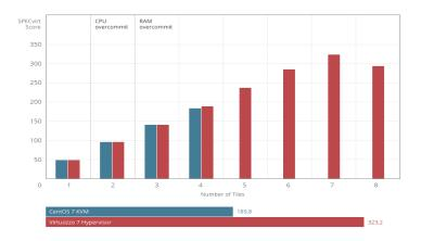
This graph depicts a SPECvirt performance test of Linux workloads for CentOS 7 KVM versus the Virtuozzo Hybrid Server Hypervisor. Tiles represent a set of workloads. A single tile deploys a number of different workloads, each of them generating output transactions. Here we measure the output total of all transactions.
