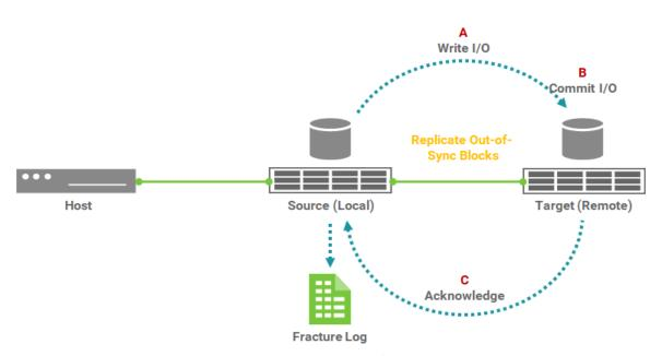
Figure 2-3 Replicate Out-of-Sync Blocks
