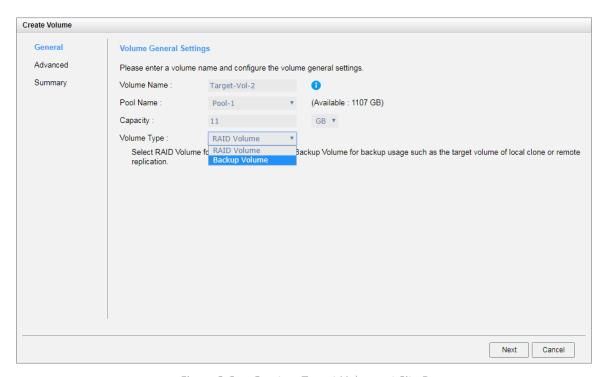
Figure 3-6 Create a Target Volume at Site B
