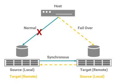
Figure 4-6 Synchronous Replication Failover
