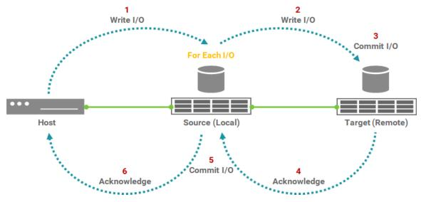
Figure 1-3 Write I/O Sequence of Synchronous Replication
