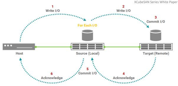
Figure 2-1 Synchronous Replication
