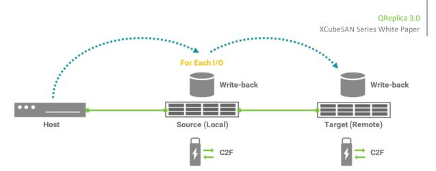
Figure 4-7 Synchronous Replication + C2F Solution
