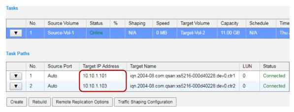
Figure 2-21 List Multipath in Remote Replication Task
