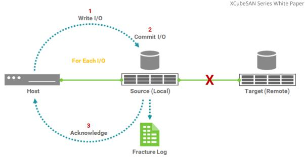
Figure 2-2 Fracture Log in Synchronous Replication
