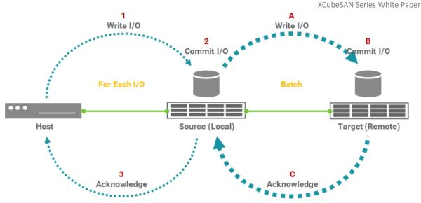
Figure 1-4 Write I/O Sequence of Asynchronous Replication
