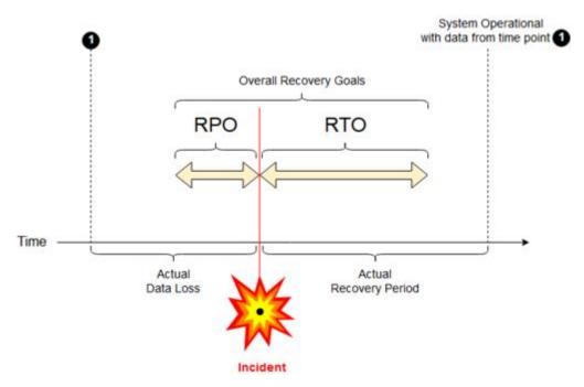
Figure 1-1 RPO and RTO Schematic Representation (from Wikipedia)
