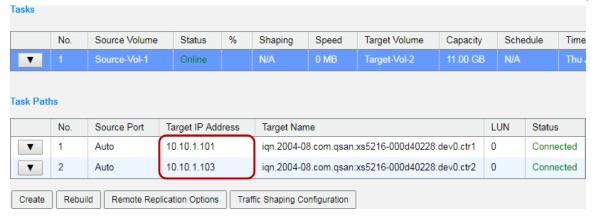
Figure 3-24 List Multipath in Remote Replication Task
