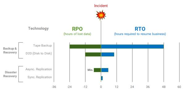
Figure 1-2 The Relationship between Backup Technologies and RPO / RTO
