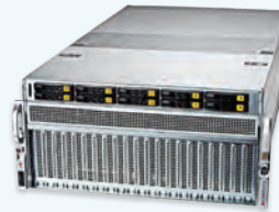
SYS-521GU-TNXR (5U) NVIDIA H100-4 5U 10 PCIe 5.0 networking slots 10x 2.5" U.2 NVMe drives Thermal capacity up 700W per GPU
